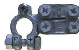
190866 Std pkg 15 A POS. 35 - 95 mm². W/ double screws and screw for aux. Tin plated.
