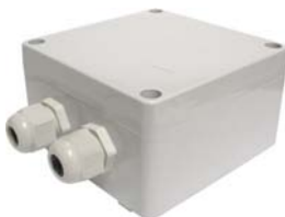
Plastic, sealed against dust and water. 6 x 8 terminals flat-plug connection. W/ locking screw. Dim.: 105 x 105 x 64 mm.
