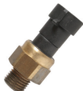
180973 A M14-1.25, 117 °C. Replacing original switch w/ yellow ring.
