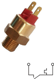
181033 M14-1.5, 102-97 °C. Jointly used w/ Cargo 181034.
