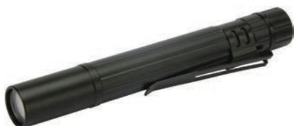
171704 LED Penlight Dim. 14.5x109 mm, Battery type AAA, Bulb type LED, Material Aluminium, No./batteries 1, Waterproof Yes, Drop proof Yes, Approvals CE Button w/ easy touch for either signal or constant light. Optical lense intensive the light. At least 8 hours of burn time.
