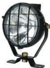
170293 Spot Light 12 V, 55 W, Light aperture 120 mm, Dim. 235x73 mm, Cable length 6000 mm, Type 1 Halogen, Type 2 H3, Socket type PK22s, Connection cable w/ Colour Black, Material/house Shockproof plastic, Shape Round, Lighter plug incl. Yes, Bulb incl. Yes, Protective cover w/, Switch w/ Hand-held.
