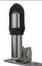
170562 Beacon Socket Mount. 2 screws, Socket DIN 72591 2 terminal, Material Galvanised steel, Bracket Angled 90°
