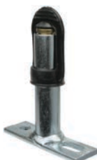
170405 Beacon Socket Mount. Flat, Length 108 mm, Mount. hole size 10 mm, Socket DIN 72591 2 terminal, Material Galvanised steel, Bracket Angled 90°
