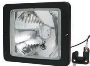
170690 Light Unit Servicing: Chrysler, Fendt, Ford, GM, IH/ Case, Isuzu, John Deere, Mazda 60/65, 75/70 W, Dim. 167x106.7 mm, Bulb type H4, Socket type P43t, Shape Rectangular, Connection Multiplug, E-approval Yes
