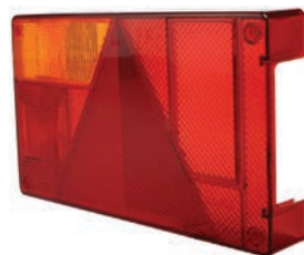
171057 Lens, Rear Lamp Servicing: Cargo 171050, 171054 Dim. 235x135x52 mm, Material Shockproof plastic, Shape Rectangular, Numberplate light w/, Reflector w/, RH/ LH LH
