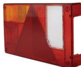
171059 Lens, Rear Lamp Servicing: Cargo 171055 Dim. 235x135 mm, Material Shockproof plastic, Shape Rectangular, Numberplate light w/, Reflector w/, RH/ LH LH
