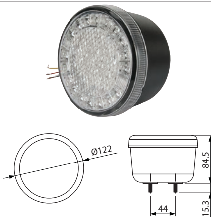
171725 LED Tail-Position Lamp 12/24 V, Dim. 122x84.5 mm, OD 122 mm, Dist. mount. holes 44 mm, Cable length 150 mm, Type LED, Material Shockproof plastic, Material/dome Shockproof plastic, Fixing screw 6, Shape Round, Connection Cable, LEDs w/, LEDs 2 44, Flasher light w/, Tail light w/, Stop light w/, Reflector w/o, E-approval Yes Ring: amber, center: red.
