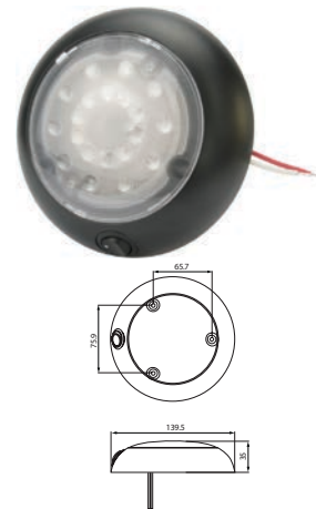
171677 LED Interior Lamp 12/24 V, 1.5 W, OD 139.5 mm, Dist. mount. holes 75 mm, Type LED, Colour Black, Material Shockproof plastic, Shape Circular, Connection Cable, LEDs w/, LEDs 2 20, Switch w/, Approvals CE, E-approval Yes
