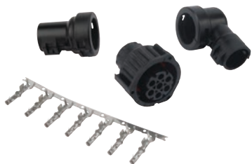
171788 Multiconnector 7 pin Servicing: Cargo 171756, 171757 Type/terminal Round, Colour Black, No./poles 7, Plug Female Gasket: Cargo 192178.
