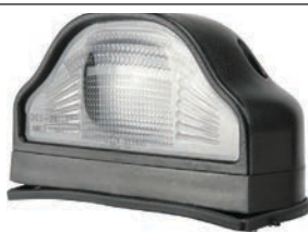
171738 LED Numberplate Lamp 24 V, Dim. 75x29x34 mm, Dist. mount. holes 65 mm, Mount. 2 screws, Cable length 300 mm, Type LED, Connection Cable, LEDs w/, LEDs 2 3, Numberplate light w/
