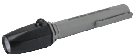
171792 LED Penlight Light power 24 lumen, Dim. 140 mm, Battery type AAA, Bulb type LED, Material Shockproof plastic, No./batteries 2, Waterproof Yes, Clips w/, Approvals ATEX Zener volt = 34-40.
