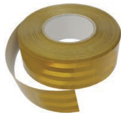
171554 Reflector Tape Dim. 50x5000 mm, Mount. Self adhesive, Colour Yellow, E-approval Yes Safety marking for heavy vehicles and trailers. Mounting on rigid surface.
