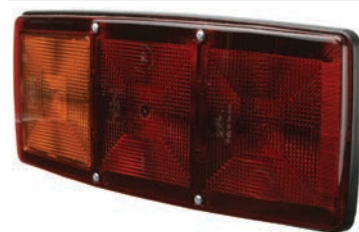
171199 Multi Function Lamp Servicing: Mercedes 21 W 1, Dim. 344x147x72 mm, Dist. mount. holes 152 mm, Socket type 1 BA15S, Material Shockproof plastic, Fixing screw 2, Shape Rectangular, Connection A, LEDs w/o, Numberplate light w/o, Flasher light w/, Tail light w/, Stop light w/, Bulb incl. No, Reflector w/o, RH/ LH RH Fits w/ Cargo 171201. Lens: Cargo 171252. More info page 98.
