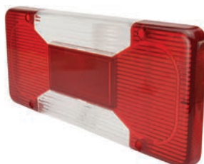
171703 Lens, Rear Lamp Servicing: Cargo 171701 Dim. 303x130 mm, Material Shockproof plastic, Shape Rectangular, Numberplate light w/o, Reflector w/, RH/ LH LH
