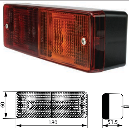
170985 Multi Function Lamp 10 W 1, 21/5 W 2, Dim. 180x60x51.5 mm, Dist. mount. holes 134 mm, Socket type 1 BA15S, Socket type 2 BAY15d, Material Shockproof plastic, Fixing screw 2, Shape Rectangular, Connection Connection, Numberplate light w/o, Flasher light w/, Tail light w/, Stop light w/, Bulb incl. No, RH/ LH RH/LH, E-approval Yes Lens: Cargo 170987.
