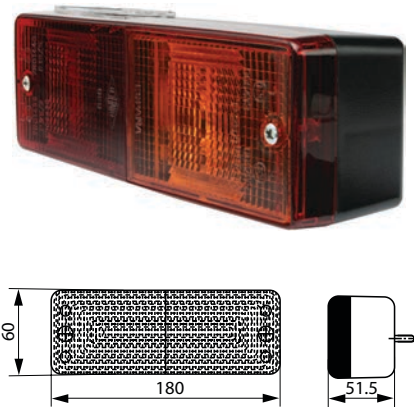
170986 Multi Function Lamp 10 W 1, 21/5 W 2, Dim. 180x60x51.5 mm, Dist. mount. holes 134 mm, Socket type 1 BA15S, Socket type 2 BAY15d, Material Shockproof plastic, Fixing screw 2, Shape Rectangular, Connection Connection, Numberplate light w/, Flasher light w/, Tail light w/, Stop light w/, Bulb incl. No, RH/ LH RH/LH, E-approval Yes Lens: Cargo 170987.
