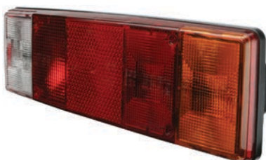
170602 Multi Function Lamp Servicing: RVI Renault, Pegaso 21 W 1, 5 W 2, 10 W 3, Dim. 406x135x74 mm, Dist. mount. holes 152 mm, Socket type 1 BA15S, Socket type 2 BA15S, Socket type 3 BA15S, Material Shockproof plastic, Shape Rectangular, Connection A, LEDs w/o, Numberplate light w/, Rear/fog lamp w/, Flasher light w/, Reverse light w/, Tail light w/, Stop light w/, Bulb incl. No, Reflector w/, RH/ LH LH, E-approval Yes Fits w/ Cargo 170603. Lens: Cargo 170665. More info page 98.
