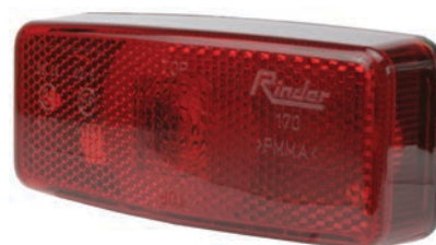
171702 Lens, Rear Lamp Servicing: Cargo 171700, 171701 Dim. 303x130 mm, Material Shockproof plastic, Shape Rectangular, Reflector w/, RH/ LH RH
