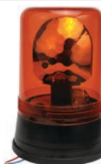
170435 Rotating Beacon 12 V, OD 160 mm, Mount. Standard ISO B2 (and B1) - Base, Height 220 mm, - Lens type PMMA/ACRYL, Bulb type H1, Model AEB TYPE 595, Colour Orange, Bulb incl. Yes, E-approval Yes Lens: Cargo 170308. Motor: Cargo 170505.
