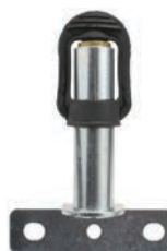
170537 Beacon Socket Mount. Vertical, Socket DIN 72591 2 terminal, Material Electro galvanized, Bracket Straight
