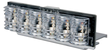
171856 LED Flash, amber Servicing: Cargo: 171849, 171850, 171852. 12 V, Length 120 mm, Height 36.75 mm, Width 18.78 mm, Bulb type 6 LED, Colour Orange
