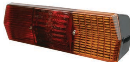
170602 Multi Function Lamp Servicing: RVI Renault, Pegaso 21 W 1, 5 W 2, 10 W 3, Dim. 406x135x74 mm, Dist. mount. holes 152 mm, Socket type 1 BA15S, Socket type 2 BA15S, Socket type 3 BA15S, Material Shockproof plastic, Shape Rectangular, Connection A, LEDs w/o, Numberplate light w/, Rear/fog lamp w/, Flasher light w/, Reverse light w/, Tail light w/, Stop light w/, Bulb incl. No, Reflector w/, RH/ LH LH, E-approval Yes Fits w/ Cargo 170603. Lens: Cargo 170665. More info page 98.
