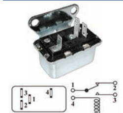
MT0533 QTY: 1 A/C Control, Blower Motor, Radiator Fan Relay w/ Resistor Normal Open - Single Pull Single Throw Voltage: 12.0 Amps: 40/30 Pigtail: MT0911 Audi Chrysler General Motors Volkswagen
