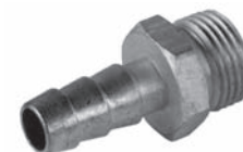
080958 Std pkg 10 Screw terminal M 18-1.5. For 10 mm. hose I.D.
