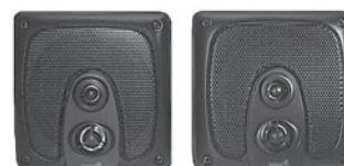
040197 Impedance 4 Ohm. Dim: 97 x 95 x 95 mm. Max. power 20/40 Watt. Supplied with mounting bracket. Supplied in pairs.
