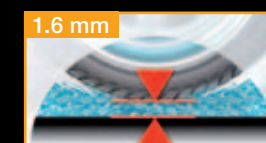
1.6 mm of tread depth Insufficient tyre tread
