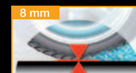
8 mm of tread depth Sufficient tyre tread
